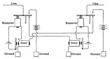
FIG. 172. Diagram of Repeater Circuits showing the principles involved but omitting detail.
